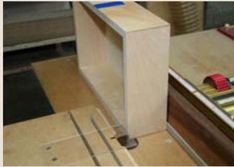
▲ Pic.2 Once the lid has been separated from the base, the sawn edges can be cleaned up using a sanding board or a spiral bit in the router table
