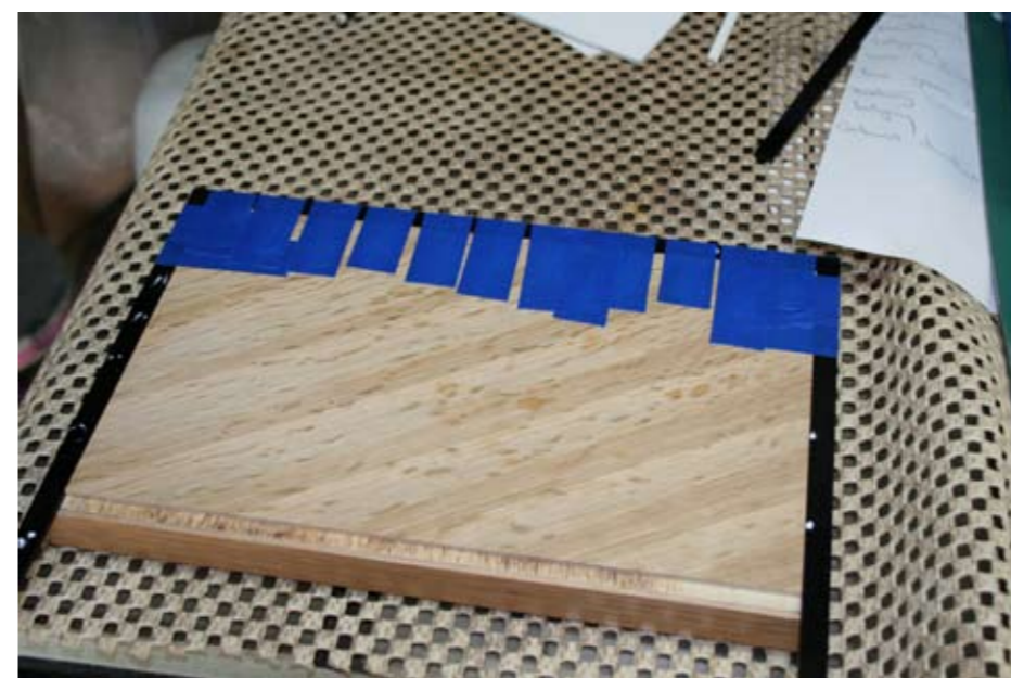
▲ Pic.4 The banding is fitted with polyurethane glue and held in place with masking tape while it dries
