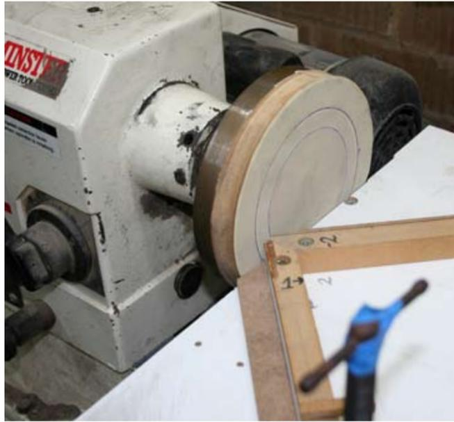
◀ Pic.3 To mitre the strips of acetal banding, Ian uses a disc sander fitted to his lathe and two mitred fences
