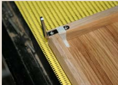
▲ Pic.5 When you've cut the hinge mortises, tape the hinges into place in the lid, then fit the lid to the base to check their alignment
