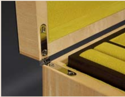
▲ Pic.1 Ian's hinges act like quadrant hinges, holding the lid open at 95°, but without any awkward mortising or clumsy stay arm
