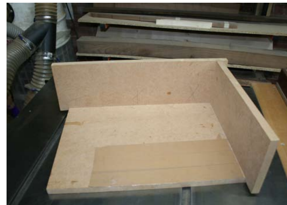
▲ Pic.2 Simple, but well worth having: a right-angled jig is a stress-free way to get your boxes square first time
