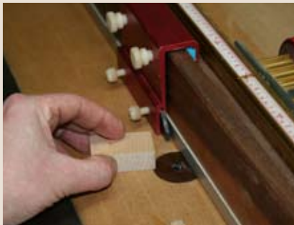
▲ Pic.4 Ian uses a block sized to match the length of the hinge mortise to set the stop on the router table fence accurately
