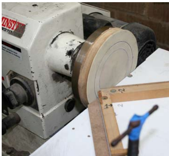
◀ Pic.3 To mitre the strips of acetal banding, Ian uses a disc sander fitted to his lathe and two mitred fences
