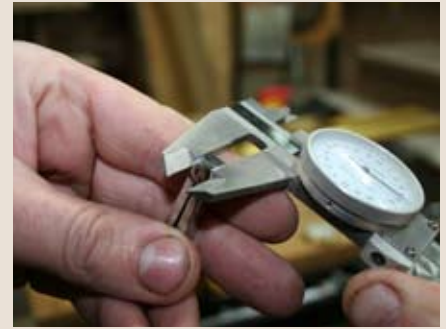
▲ Pic.3 Measure the barrel of the closed hinge and divide by two to determine the depth of cut necessary to house it in the base and lid
